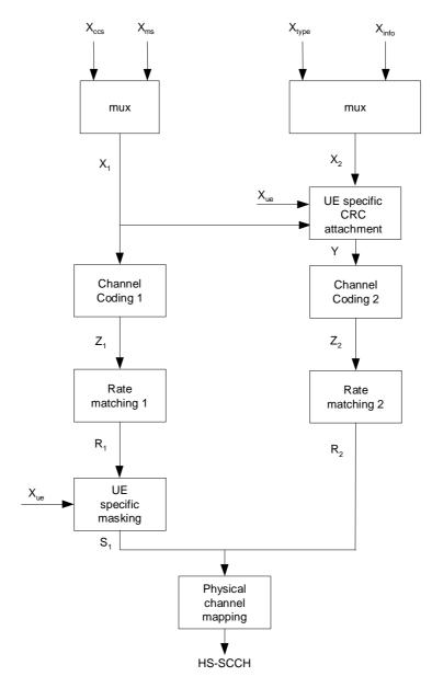
Figure 19A: Coding chain for HS-SCCH type 2
